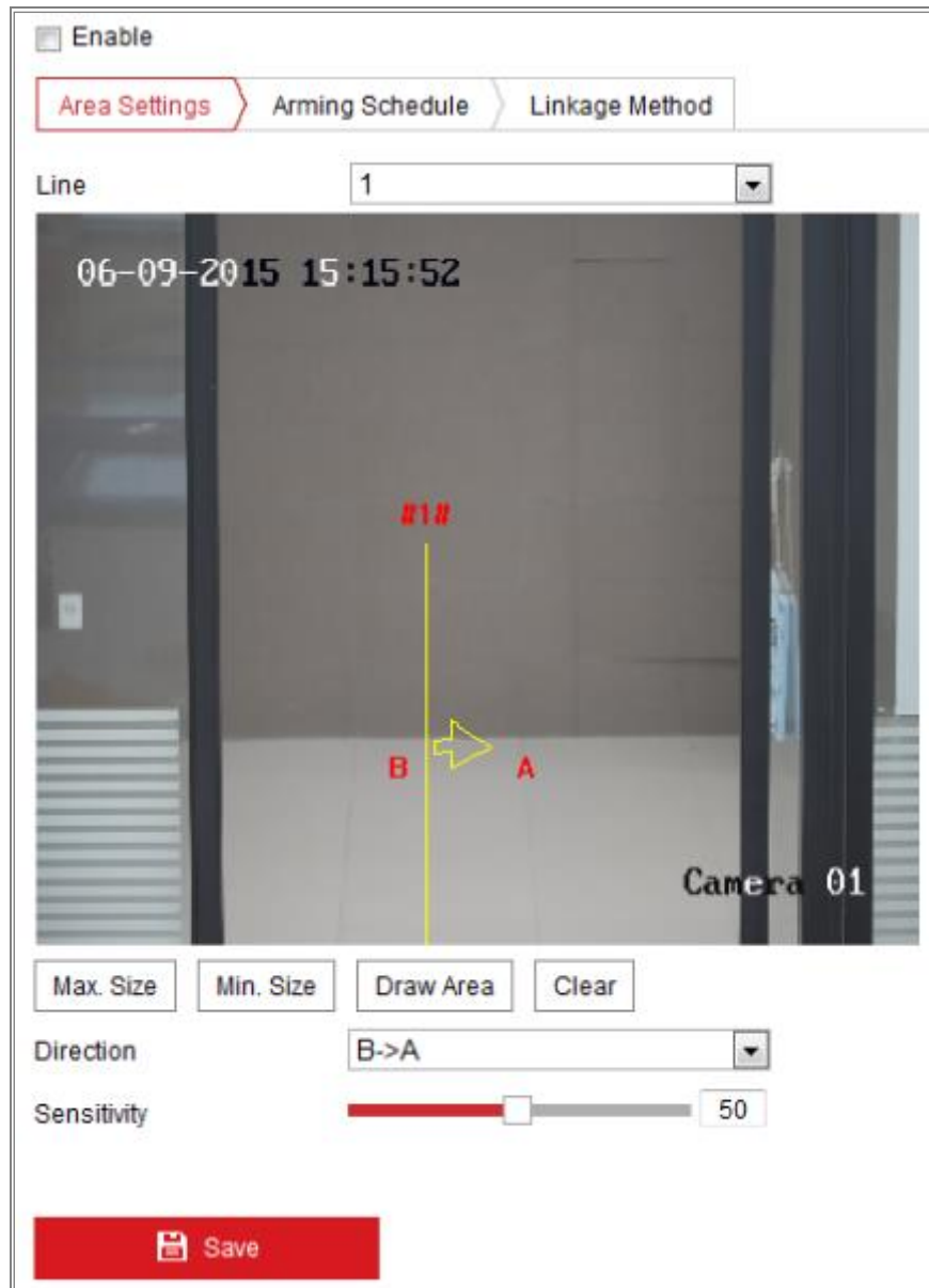
Figure 10-20 Line Crossing Detection
