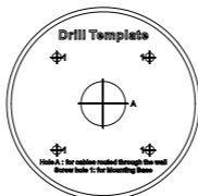
Figure 2-12 Drill Template of the Junction Box
