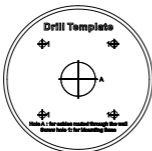
Figure 2-15 Drill Template of the Junction Box
