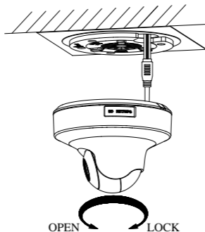
Figure 2-4 Connect the Cables
